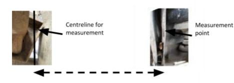
Must be a minimum of 50mm between front and any support bar. No gusset bars between front and support with the exception of angle style from main rail to bumper as shown.
