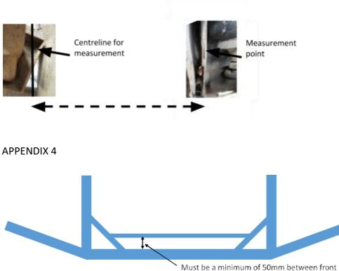
Must be a minimum of 50mm between front and any support bar. No gusset bars between front and support with the exception of angle style from main rail to bumper as shown.
